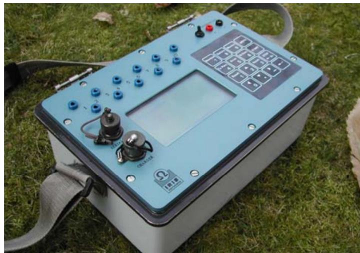
Figura 1.7: Imagem do receptor ELREC PRO (IRIS INSTRUMENTS. <http://www.iris-instruments.com/ELRECPRO.pdf>, 18 jan. 2014).
