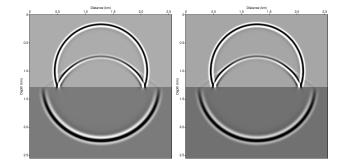
Impulse response for the two layer model based on the solution of: Coupled wave equation system (left); First-order wave equation; (right)
