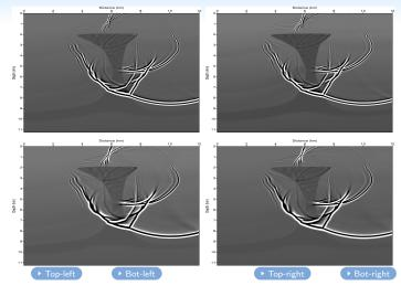
Coupled wave equation system; (top left); First-order wave equation; (top right); Modified Chebyshev polynomials (bottom left); and the REM (bottom right)
