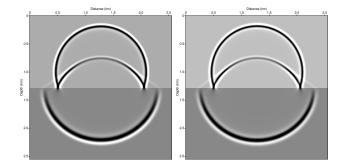
Impulse response for the two layer model based on the solution of: Modified Chebyshev polynomials (left); The REM (right)
